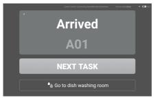
6. The "Arrived at task point" interface is the same as the "Call arrival" interface, the user needs to judge whether the next task can be performed or return directly based on the remaining space of the robot currently loaded
