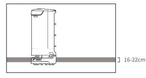
7. The ceiling height is within the range of 2-8 meters (higher or lower may require technical evaluation); taking the height of 3 meters as an example, it is necessary to apply a graphic mark every 2 meters or so, there is no lighting fixture or other strong light source in the 30cm area around the graphic mark. (Data for specific interval needs to be provided by Technology Dept.)
