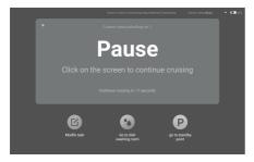
4. During the cruise process, you can touch the robot screen to stop the command, and the robot will stop for waiting immediately, if a touch command is not received after 10 seconds, the robot will continue to perform the task.
