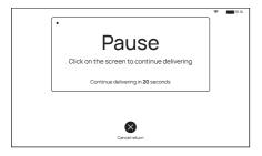
4. During the cruise process, you can touch the robot screen to stop the command, and the robot will stop for waiting immediately, if a touch command is not received after 20 seconds, the robot will continue to perform the task.
