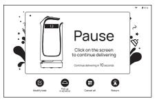
5. The robot quickly arrives at the designated location according to the established trajectory. During the delivery process, you can touch the robot screen to stop the command, and the robot will stop for waiting immediately, if a touch command is not received after 5 seconds, the robot will continue to perform the task. After the pause, the screen enters this interface, you can perform operations such as modifying the task, bringing food in advance, canceling all tasks, and returning.
