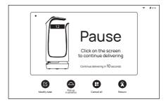
4. During the motion process, you can click the robot screen, and the robot will stop for waiting immediately, if a touch command is not received after 20 seconds, the robot will continue to perform the task. 5. After reaching the destination, return to the main interface of the direct delivery mode, select a destination, and the robot can proceed with the next task.
