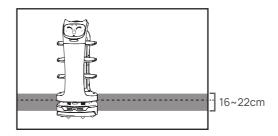
7. The ceiling height is within the range of 2-8 meters (higher or lower may require technical evaluation); taking the height of 3 meters as an example, it is necessary to apply a graphic mark every 2 meters or so, there is no lighting fixture or other strong light source in the 30cm area around the graphic mark. (Data for specific interval needs to be provided by Technology Dept.)
