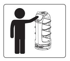
5. When picking up the food, please stand in front of the robot or touch the robot display screen, the robot stops running, and the screen enters the pause page, indicating that the robot stops running, and the diners can pick up food at will.
