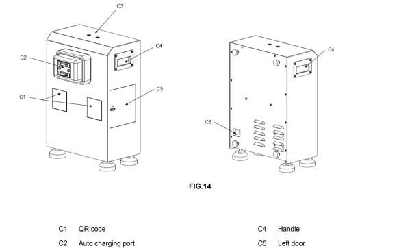
There is an output power cord located behind the left door (C5) for manual charging. This function can be used when the battery is in dormant mode or needs manual charging.
